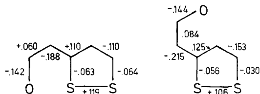
Fig. 5. Calculated changes in \pi -bond order \delta p_{\mu\nu} = p_{\mu\nu}^* - p_{\mu\nu}^0 for I and VI according to a PPP-calculation
